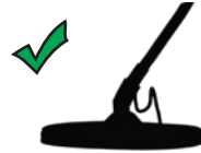
Correct search coil angle
