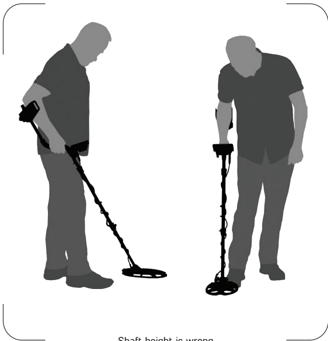
Shaft height is wrong
